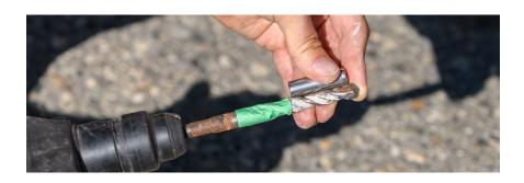
Drill all holes to the depth indicated by the tape or marker applied to the drill in step 4. Holes must be vertical to properly anchor the product.
